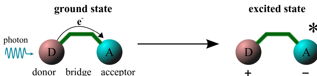
Figure 2.2: Photoinduced intramolecular charge transfer (ICT) in a donor-acceptor molecule
